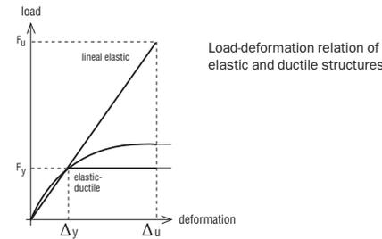
The toughness of the structure – the so called ductility (non-linear deformation capacity) – improves the load bearing performance of timber structures under earthquake loading. The ductile deformation capacity helps the structure to dissipate energy.
