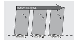
Overturning forces (compression and tensile forces)
