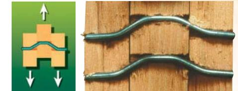
The plastic deformation results from the ductile behaviour of the fasteners and the local plastification of the wood.
