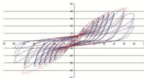
Load-deformation of a shear wall under cyclic loading
