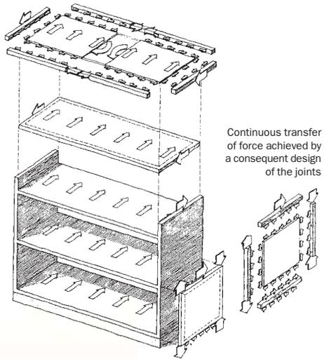
The earthquake movements cause inertia loads which magnitude depends amongst others on the moving mass. In most cases, only horizontal inertia loads are relevant for the design.
