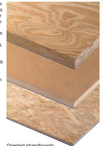
Fibreboards are built-up from lignified fibres pressed together partly with added adhesives.
