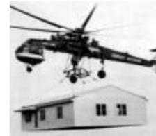
Wood has a better proportion of strength to dead load than other construction materials. The light weight of wood-frame buildings causes smaller inertia forces and results in a comparatively smaller design loads.
